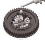
Fill the space around the gears with the indicated Serpent Diff Oil **until level with the top of the casing**. Rotate the output shaft to allow the grease to fill all gaps in and around the gears.
