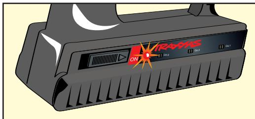
4. Turn on the transmitter and check the power indicator for a solid red light.
