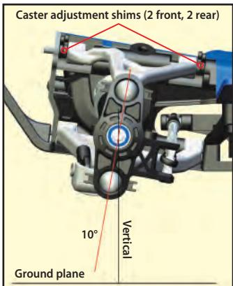
page 43, and look up your caster angle setting to find the correct position for the outer toe links. Positioning the toe-links correctly will maintain the original factory geometry and eliminate the unwanted steering angle changes caused by bump steer.
