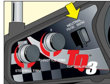
50/50 is the required setting for Revo with the TRX 3.3 Racing Engine.
