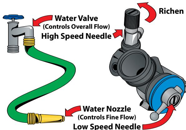
is increased, the low-speed needle is pulled completely away from the needle seat leaving it fully open. At that point, fuel metering is entirely controlled by the high-speed needle. Again, using our water hose example, when the spray nozzle at the end of our garden hose is fully open, then the main water valve can be used to adjust how fast the water flows.
