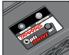
The OptiDrive module prevents the transmission from changing directions while the truck is in motion. The truck must be completely stopped to change directions, regardless of the position of the shift selector switch on the transmitter. The OptiDrive module is preset at the factory. If the transmitter throttle trim adjustment is changed, then the OptiDrive module will need to be re-programmed.
