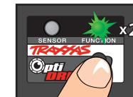
4. Pull the transmitter throttle trigger to the full throttle position. Hold it there until the Function LED flashes green three times. **Note:** The throttle servo will not move during programming even though it is connected to the controller.
