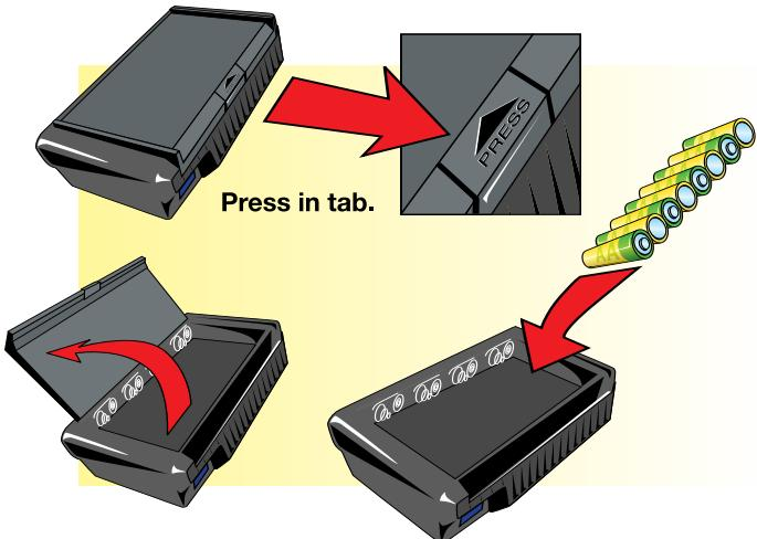
1. Remove the battery compartment door by pressing the tab and lifting the door up.
