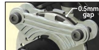
1. Use a .50mm feeler gauge between the brake pad insert and brake disk.
