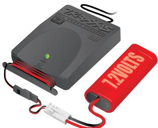
5. **1500mAh or lower capacity:** When the light turns solid green (not flashing), the battery pack is fully charged and ready for use.
