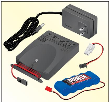
To power the radio system in the truck, your Revo is equipped with the RX Power Pack, a rechargeable 5-cell nickel metal hydride (NiMH) battery pack. The RX Power Pack must be fully charged before running the truck. The supplied TRX Power Charger is a peak-detecting unit that will charge the supplied RX Power Pack in about one hour. The peak-detection
