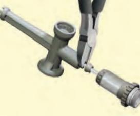
C. Remove/Install Rod End
