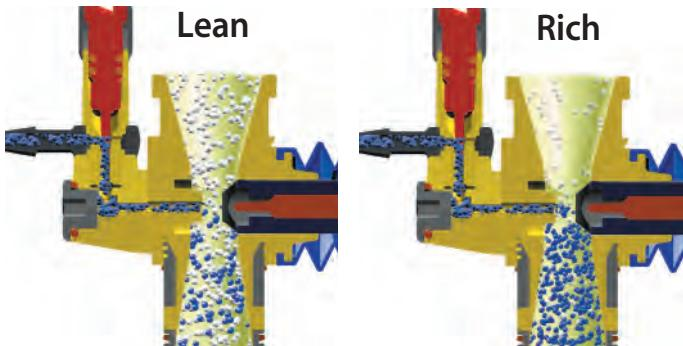
© Slightly lean fuel mixtures deliver stronger, more efficient combustion and more power, but with less lubrication.
