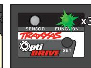
5. Release the transmitter throttle trigger allowing it to return to neutral. The Function LED will turn solid green, indicating that the shifting servo is OK to shift and the programming has been completed. The controller is now programmed and ready to go!
